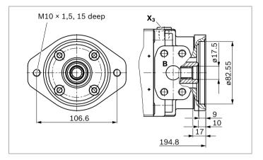
▼ K02: Flange 101-2 (B), hub for splined shaft 7/8 in (22-4)
